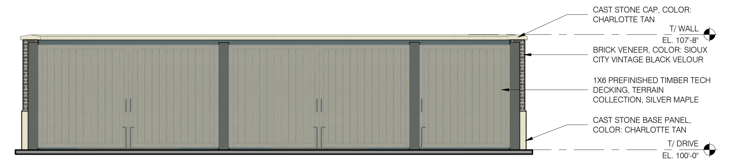
5 FRONT DUMPSTER ELEVATION SCALE: 1/4" = 1'-0"
